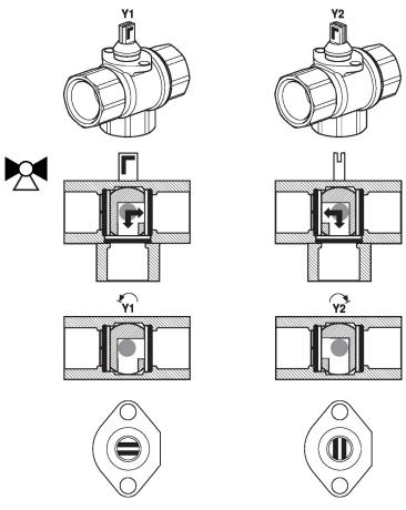
**Flow setting** At the actuator the end stop clip has to be removed in order to get the angle of rotation of 90°, which is needed for the change-over functionality.
